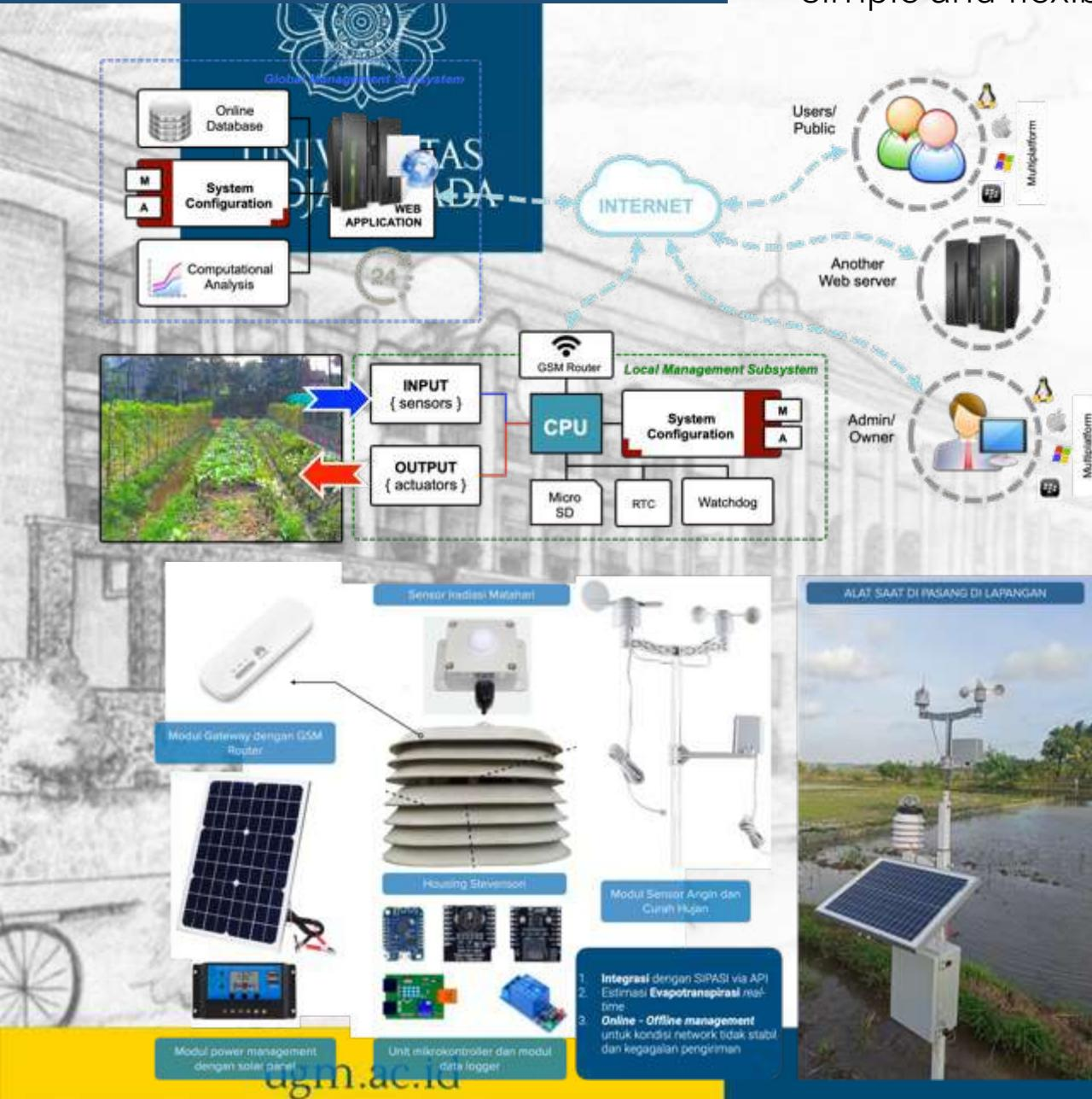
The framework utilizes **local** and **global** subsystem to establish a simple and flexible environmental **monitoring** and **control**
